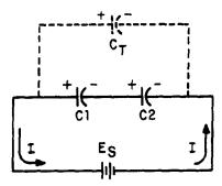
Figure 3-13.—Capacitors in series.
