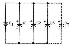
Figure 3-14.—Parallel capacitive circuit.
