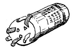
Figure 3-18.—Construction of an electrolytic capacitor.
