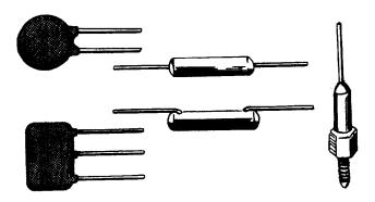
Figure 3-17.—Ceramic capacitors.
