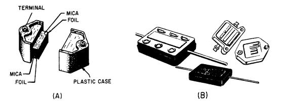
Figure 3-16.—Typical mica capacitors.
