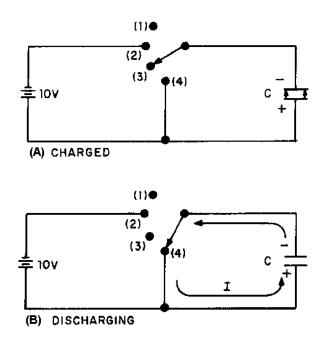
Figure 3-8.—Discharging a capacitor.
