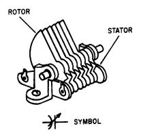
Figure 3-19.—Rotor-stator type variable capacitor.
