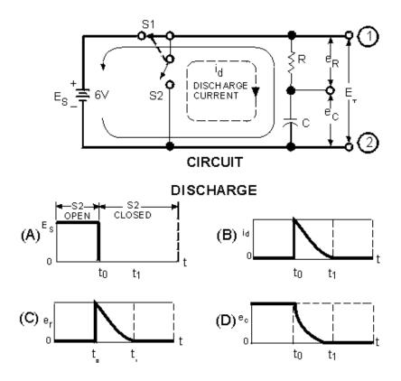
Figure 3-10.—Discharge of an RC Series circuit.
