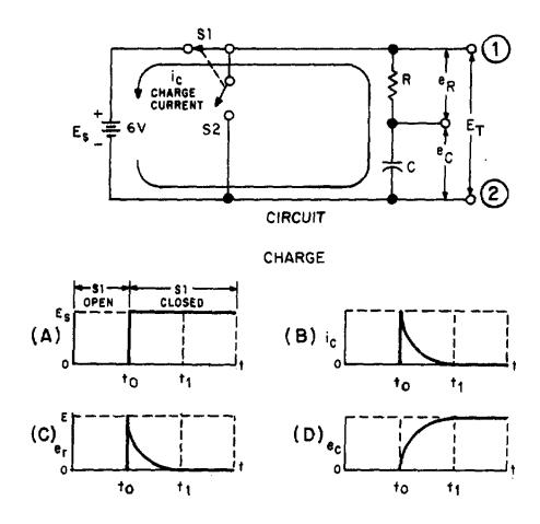
Figure 3-9.—Charge of an RC series circuit.
