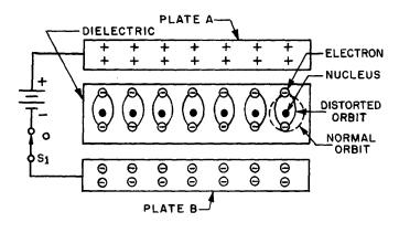
Figure 3-4.—Distortion of electron orbits in a dielectric.
