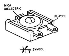
Figure 3-20.—Trimmer capacitor.
