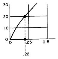
The value selected from the graph means that a capacitor (including the one you are solving for) will reach twenty percent of full charge in twenty-two one hundredths (.22) of one RC time constant. Remember that it takes  $100~\mu s$  for the capacitor to reach 20% of full charge. Since  $100~\mu s$  is equal to .22 RC (twenty-two one-hundredths), then the time required to reach one RC time constant must be equal to:
