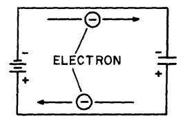
Figure 3-7.—Electron motion during charge.
