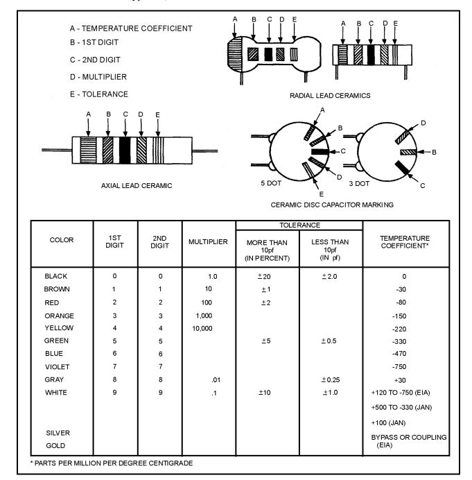
Figure 3-23.—Ceramic capacitor color code.
