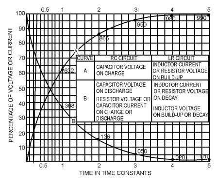
Figure 3-12.—Universal time constant chart for RC and RL circuit.
