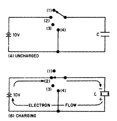
Figure 3-6.—Charging a capacitor.
